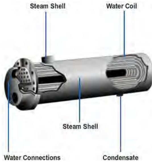
Figure 10-21 - Instantaneous-type water heater.
