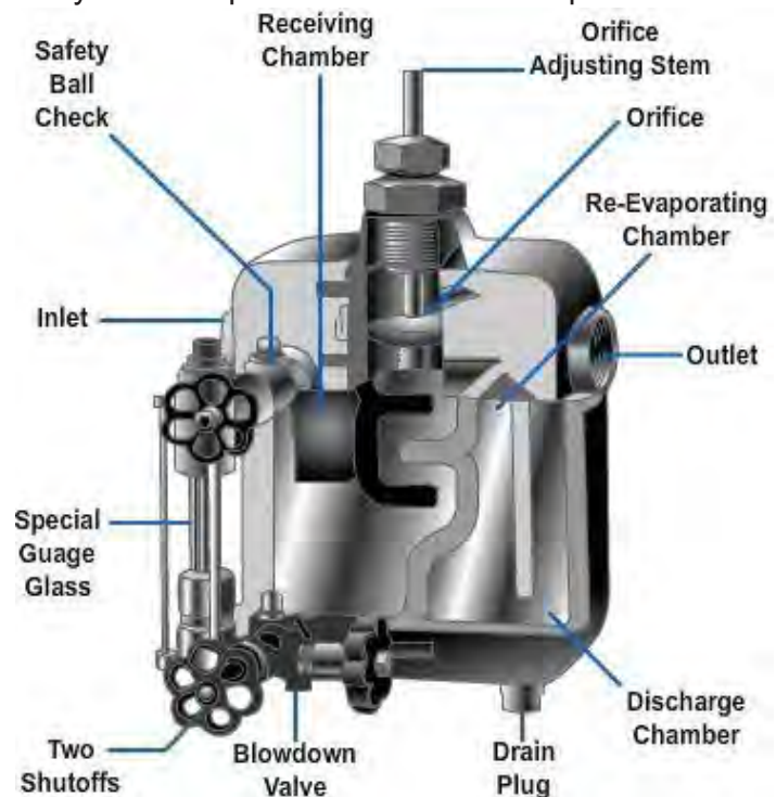
Figure 10-17 – Throttling trap.
